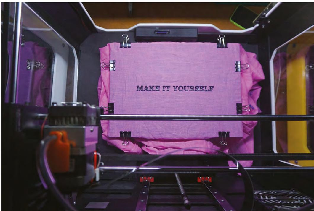
**Left** ■ We attached the fabric securely with clips on all sides. It must be as taut as possible
